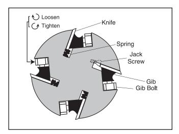
**Figure 43.** Cutterhead profile diagram.
